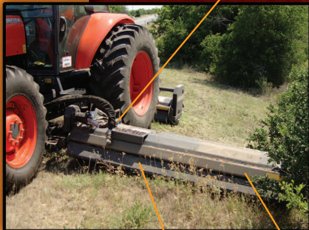
Full width front metal guarding & rear debris deflector
