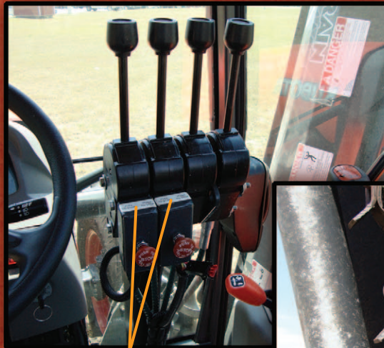
Integrated, ignition lock-out prevents the tractor from starting with the wing cutting head(s) engaged
