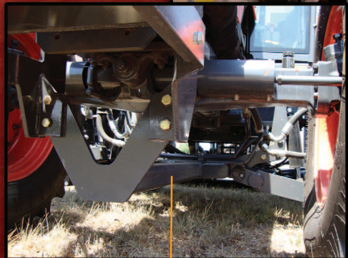
Full length subframe mounted from the front bolster to the rear axle
