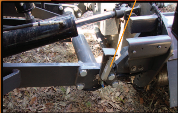
Automatic wing shut-off in raised position
